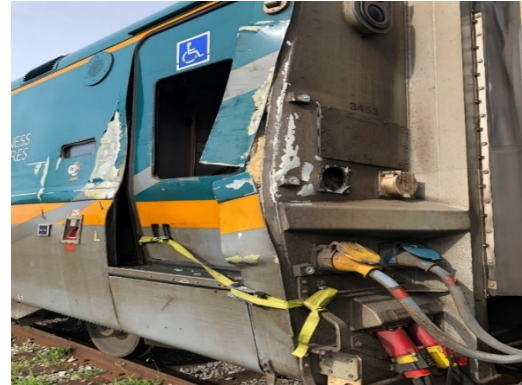
Figure 4. Damaged business LRC car of VIA 48 (Source: VIA Rail Canada Inc.)
