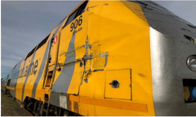
Figure 3. Damaged lead locomotive of VIA 48 (Source: VIA Rail Canada Inc.)
